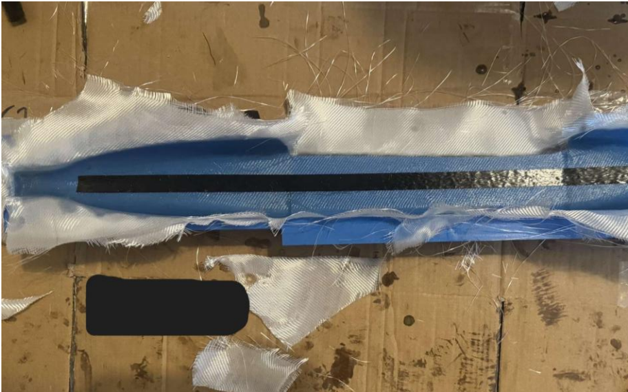
Lay-up of one side of the fuselage ready to be vacuum sealed. The black strip is Carbon Tow tape, providing localised extra strength in bending.
