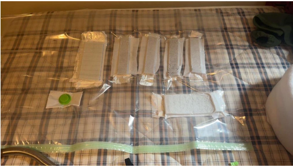
Initial aerofoil prototypes using various plies and combinations of 100gsm 2x2 twill and 320gsm Biaxial fibre.
