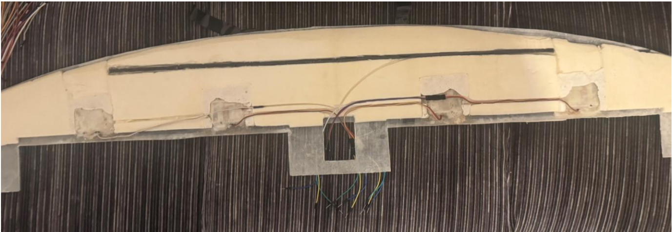
Lay-up of one side of the fuselage ready to be vacuum sealed. The black strip is Carbon Tow tape, providing localised extra strength in bending.
